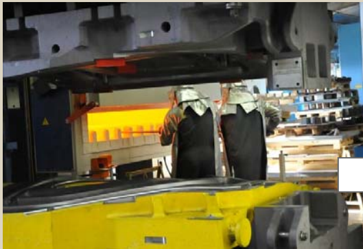
Austenitization (heating) of blanks
