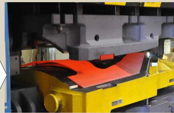
Hot forming + die quenching
